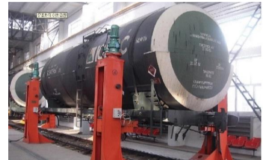
Changing wheels (standard · broad gauge) by lifting the train body
